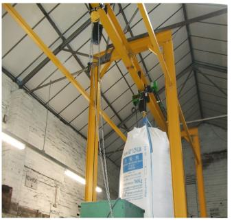
Fixed Gantry cranes are the perfect crane in situations where a load needs to be moved in a single axis once lifted. The runway beam which the hoist runs can be formed into bends to allow the hoist to go around corners.
